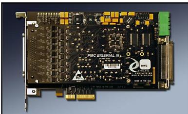
Couple a Dynamic Engineering PCIe carrier with any of our PMC boards. Carriers available in 1 and 4 lane configurations. See a full list of [PMC](#) solutions below.
