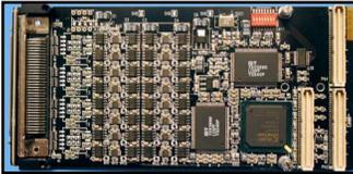
**PMC Compatible Bi-Directional Serial Data Interface**
