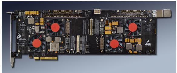
Shown With JN4 full CB, 4 fans installed, AP power connector
