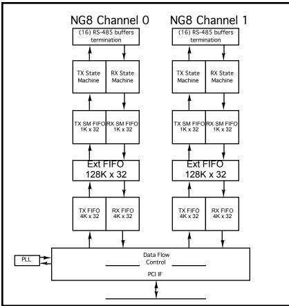
Figure 1 PMC-BISERIAL-III-NG8 Block Diagram
