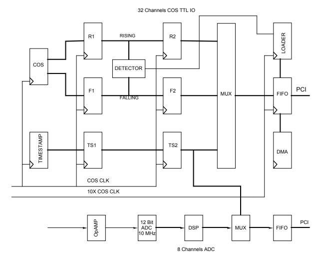
Figure 2 ccPMC-PARALLEL-TTL-BA18 Operational Block Diagram
