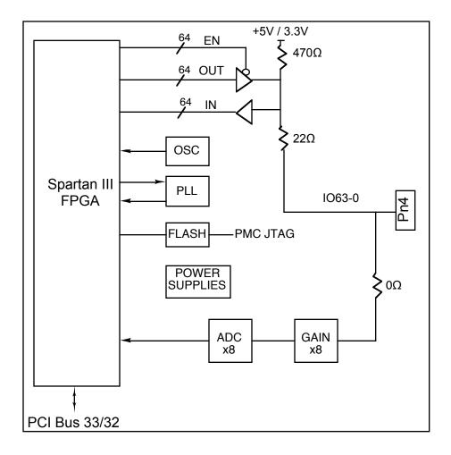
Figure 1 ccPMC-PARALLEL-TTL Block Diagram
