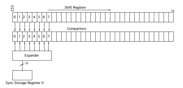
Verbose Sync mode requires a sync pattern. The pattern is stored into the Sync Register File for COM1/2 – address offset 7 for the channel. The register file has 8 registers of which the first 4 align with the sync pattern to be checked for. The last 4 are currently spares and can be used for future expansion. The actual number of bits used in the sync pattern is programmable via VerboseSyncEn.
